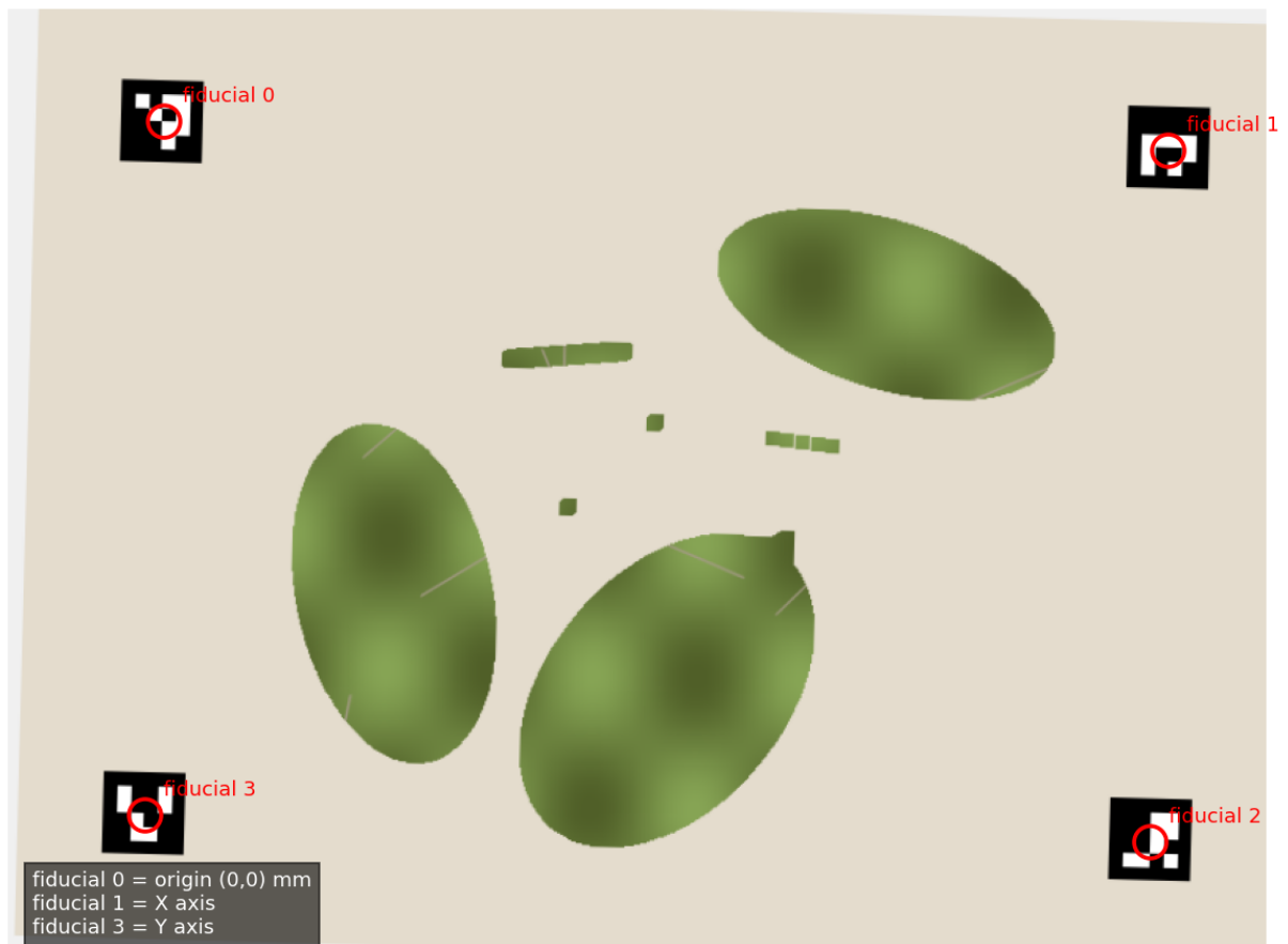
Figure 4. The sheet frame. Four ArUco fiducials at the corners of the sheet define a millimetre coordinate system: fiducial 0 is the origin, fiducial 1 defines the X axis and fiducial 3 defines the Y axis.
